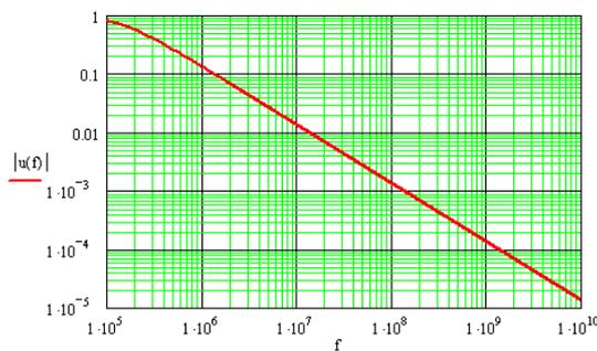
Figure 2 : Response of the integrator alone (output voltage / input voltage)
