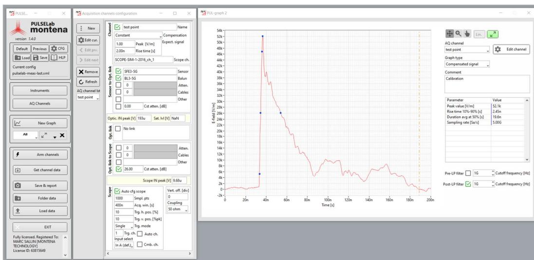
PULSELab improves the measurement accuracy by considering the transfer function of all devices used in the measurement chain (sensor, balun, attenuators, cables, fiber-optic links, etc.) and compensates the signals received by the oscilloscope to display the measured value in its own units. The correction factor of each component can be either a constant value or a frequency dependant transfer function.
