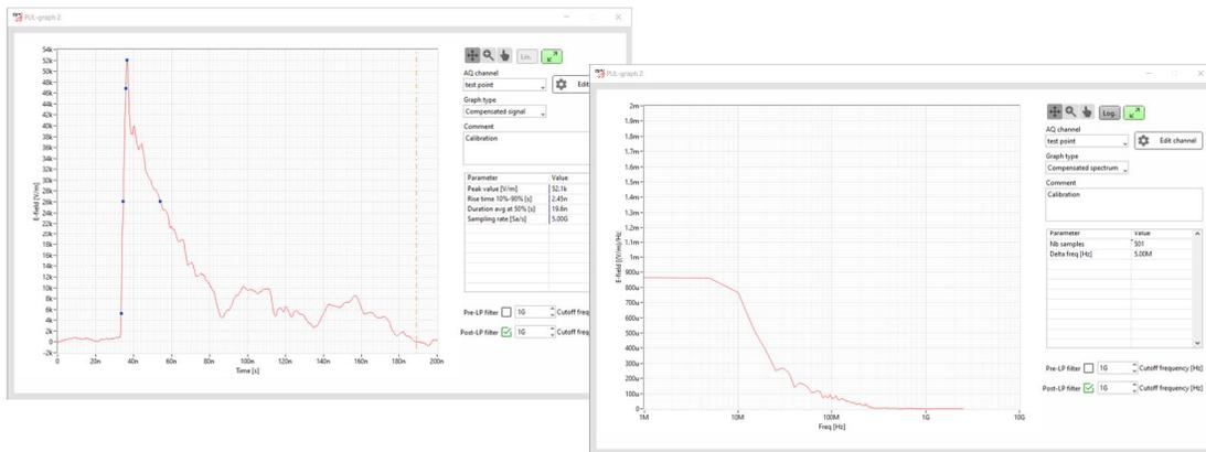
The transfer functions of all montena pulse measurement devices (sensors, baluns, fiber-optic links, ...etc) are preconfigured. The user can create and edit additional components. A more straightforward compensation approach (using constant factor and time-domain integration) can be used too.
