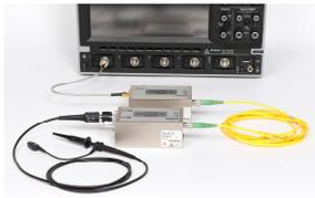
The shielded optical transmitter has a 1 M $\Omega$  / 50  $\Omega$  BNC input which enables connecting any sensing device (current probe, HV probe or specific means for HF measurements). It also makes an ideal oscilloscope front-end for the remote measurement of floating potentials in industrial applications and ensures a total galvanic insulation of the operator, for safe operation in high voltage areas.
