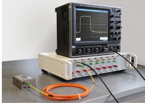
Montena MOL500T optical link is designed for real-time measurement of electric signals from DC up to 500 MHz in harsh electromagnetic environment.
