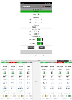
The system is delivered with montena FibREmote software for PC and Android devices. The applications allow simple configuration and monitoring of the optical link(s).
