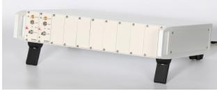
The MOL-MF-10 is a 19" 2U chassis for up to ten plug-in receiver modules. The receiver modules are powered and controlled from the chassis backplane.
